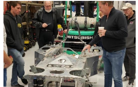
Mike telling us about safety changes to the Gurney Eagle Chassis fuel cells and the effect on the car's handling.
