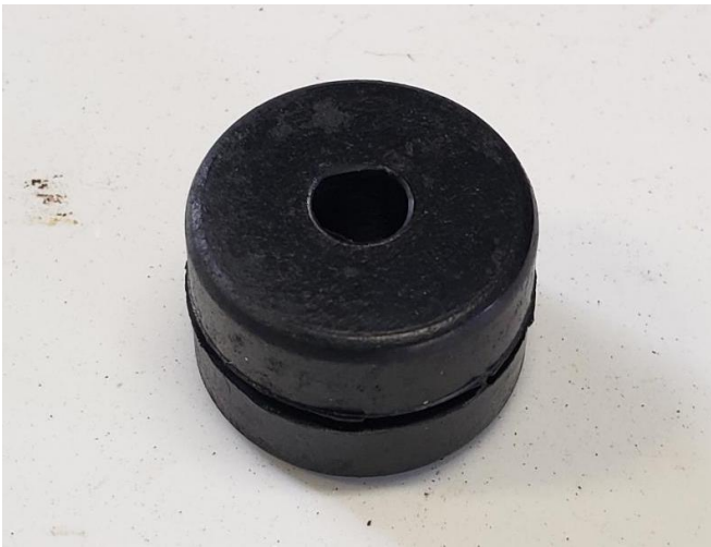
This is what the bushing for the wiper motor is supposed to look like. His motor was 'wobbling'.
