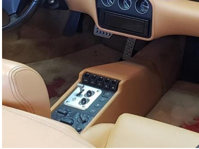
Notice the shift lever on Jim's Ferrari. It's only for selecting reverse. (BH)
