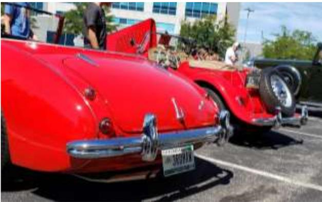
The BMC cars shared parts bins. The MG TD owner noticed the overrides on the rear bumpers of the TD and the 3000 were the same.
